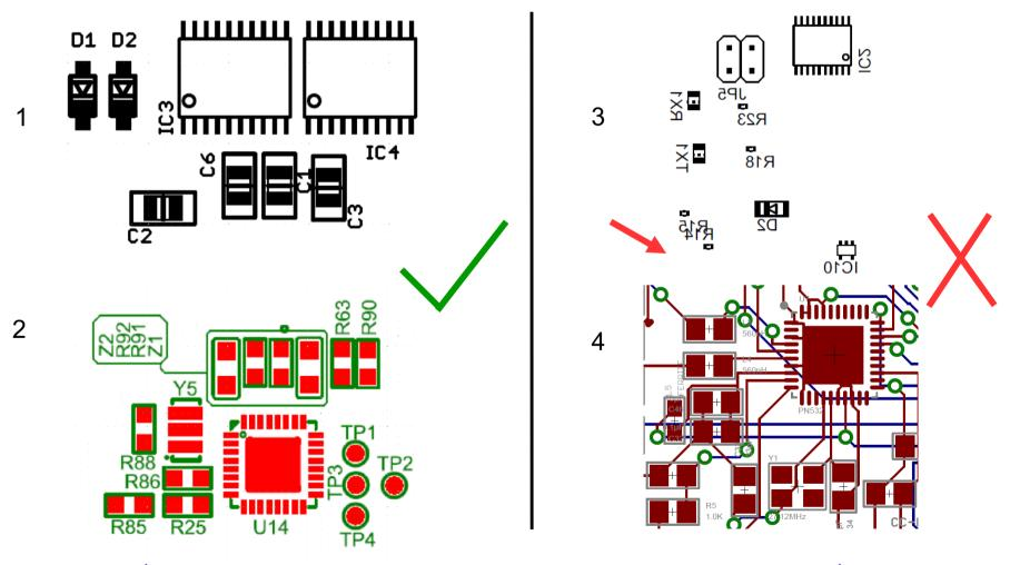
(1 and 2 is clear and good for PCBA. 3 and 4 is not clear enough for PCBA)
